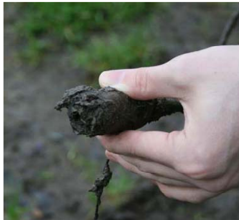
2. The mud will not cause damage to the expanded beam insert. A butt-contact connector would almost certainly already be destroyed in this state
