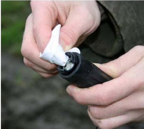
5. The insert face is dried and wiped clean. Ideally a clean cloth or tissue is used but if these are not available the bottom of your coat will suffice.
